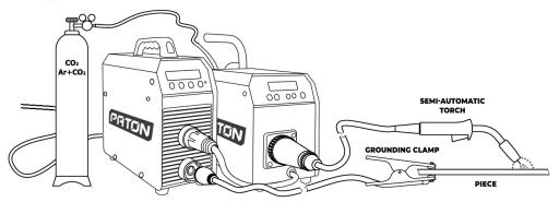
**Caution!** When welding ferrous metals, in the simplest case, carbon dioxide "CO2" is used as a shielding gas, and when welding aluminium – only inert gases such as argon "Ar", sometimes helium "He", are suitable. Alternatively, for stainless and high-alloy steels, mixtures in various proportions "80% Ar+20% CO2" are often used. Use of other gases is allowed only in agreement with the equipment manufacturer.
